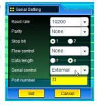
Setting for controlling the projector from the serial controller connected to the serial port.
